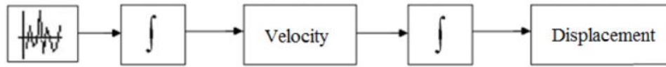
Figure 6. Scheme to obtain the velocity and displacement of the free tip of the beam.
