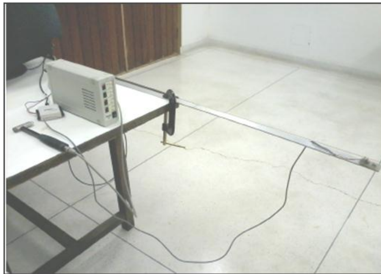
Figure 5. Experiment mounted with a cantilever beam.
